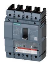
circuit breaker 3VA6 UL frame 250 breaking capacity class H 65kA @ 480V 4-pole, line protection ETU320, LI, In=250A overload protection Ir=100A...250A short-circuit protection Ii=1.5...10 x In N conductor protection adjustable (OFF, 50%, 100%) without connection
