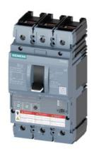
Circuit breaker 3VA6 UL frame 250 breaking capacity class H 65kA @ 480 V 3-pole, Line protection ETU320, LI, In=250A overload protection, 100% rated Ir=100A ...250A Short-circuit protection Ii=1.5...10 x In cable connection on both sides
