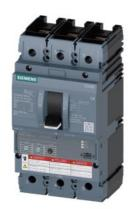
circuit breaker 3VA6 UL frame 250 breaking capacity class H 65kA @ 480 V 3-pole, line protection ETU320, LI, In=250A overload protection Ir=100A ...250A short-circuit protection Ii=1.5...10 x In nut keeper kit on both sides
