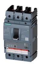
circuit breaker 3VA6 UL frame 250 breaking capacity class H 65kA @ 480V 3-pole, line protection ETU320, LI, In=250A overload protection Ir=100A...250A short-circuit protection Ii=1.5...10 x In without connection
