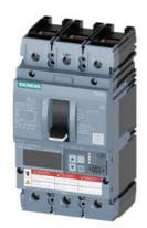
Circuit breaker 3VA6 UL frame 250 breaking capacity class M 35kA @ 480 V 3-pole, Line protection ETU856, LSI, In=250A overload protection, 100% rated Ir=100A ...250A Short-circuit protection Isd=0.6..10x In, Ii=1.5..10x In N conductor protection optionally with external CT; up to 160% Ground-fault alarm message via EFB300 or COM cable connection on both sides
