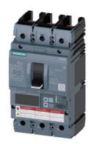
Circuit breaker 3VA6 UL frame 250 breaking capacity class M 35kA @ 480V 3pole, Line protection ETU856, LSI, In=250A overload protection, 100% rated Ir=100A...250A Short-circuit protection Isd=0.6..10x In, Ii=1.5..10x In N conductor protection optionally with external CT, up to 160% Ground-fault alarm message via EFB300 or COM without connection
