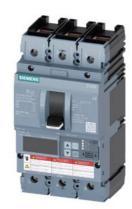
circuit breaker 3VA6 UL frame 250 breaking capacity class M 35kA @ 480 V 3-pole, line protection ETU850, LSI, In=250A overload protection Ir=100A ...250A short-circuit protection Isd=0.6..10x In, Ii=1.5..10x In N conductor protection opt. w. ext. CT; up to 160% cable connection on both sides
