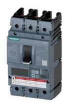
Circuit breaker 3VA6 UL frame 250 breaking capacity class M 35kA @ 480V 3pole, Line protection ETU850, LSI, In=250A overload protection, 100% rated Ir=100A...250A Short-circuit protection Isd=0.6..10x In, Ii=1.5..10x In N conductor protection optionally with external CT, up to 160% without connection
