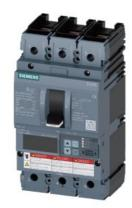
Circuit breaker 3VA6 UL frame 250 breaking capacity class M 35kA @ 480 V 3-pole, Line protection ETU830, LIG, In=250A overload protection, 100% rated Ir=100A ...250A Short-circuit protection Ii=1.5...10 x In Ground-fault protection Ig=0.2... 1 x In, tg=0.05-0.8s nut keeper kit on both sides
