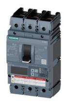
circuit breaker 3VA6 UL frame 250 breaking capacity class M 35kA @ 480 V 3-pole, line protection ETU830, LIG, In=250A overload protection Ir=100A ...250A short-circuit protection Ii=1.5...10 x In ground-fault protection Ig=0.2... 1 x In, tg=0.05-0.8s nut keeper kit on both sides
