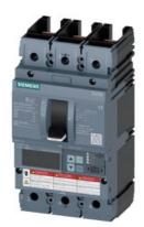
circuit breaker 3VA6 UL frame 250 breaking capacity class M 35kA @ 480V 3-pole, line protection ETU830, LIG, In=250A overload protection Ir=100A...250A short-circuit protection Ii=1.5...10 x In ground-fault protection Ig=0.2...1 x In, tg=0.05-0.8s without connection
