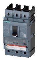
Circuit breaker 3VA6 UL frame 250 breaking capacity class M 35kA @ 480V 3-pole, Line protection ETU350, LSI, In=250A overload protection, 100% rated Ir=100A...250A Short-circuit protection Isd=1.5...10 x Ir, Ii=10 x In without connection
