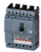
Circuit breaker 3VA6 UL frame 250 breaking capacity class M 35kA @ 480V 4pole, Line protection ETU330, LIG, In=250A overload protection, 100% rated Ir=100A...250A Short-circuit protection li=1.5...10 x In N conductor protection adjustable (OFF, 50%, 100%) Ground-fault protection Ig=0.2...1 x In= tg=0.1/0.3s without connection
