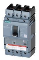
circuit breaker 3VA6 UL frame 150 3-pole, starter protection ETU310M, I, In=110A without overload protection short-circuit protection li=3...15 x In cable connection on both sides
