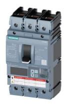
Circuit breaker 3VA6 UL frame 250 breaking capacity class C 100kA @ 480 V 3-pole, Line protection ETU856, LSI, In=100A overload protection, 100% rated Ir=40A ...100A Short-circuit protection Isd=0.6..10x In, Ii=1.5..12x In N conductor protection optionally with external CT; up to 160% Ground-fault alarm message via EFB300 or COM cable connection on both sides
