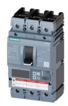
circuit breaker 3VA6 UL frame 250 breaking capacity class C 100kA @ 480 V 3pole, line protection ETU856, LSI, In=100A overload protection Ir=40A ...100A short-circuit protection Isd=0.6..10x In, Ii=1.5..12x In N conductor protection opt. w. ext. CT; up to 160% ground-fault alarm message via EFB300 or COM cable connection on both sides
