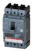
Circuit breaker 3VA6 UL frame 250 breaking capacity class C 100kA @ 480 V 3-pole, Line protection ETU856, LSI, In=100A overload protection, 100% rated Ir=40A ...100A Short-circuit protection Isd=0.6..10x In, Ii=1.5..12x In N conductor protection optionally with external CT; up to 160% Ground-fault alarm message via EFB300 or COM nut keeper kit on both sides
