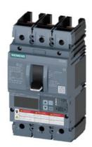
Circuit breaker 3VA6 UL frame 250 breaking capacity class C 100kA @ 480V 3-pole, Line protection ETU856, LSI, In=100A overload protection, 100% rated Ir=40A...100A Short-circuit protection Isd=0.6..10x In, Ii=1.5..12x In N conductor protection optionally with external CT, up to 160% Ground-fault alarm message via EFB300 or COM without connection
