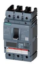
circuit breaker 3VA6 UL frame 250 breaking capacity class C 100kA @ 480V 3-pole, line protection ETU856, LSI, In=100A overload protection Ir=40A...100A short-circuit protection Isd=0.6..10x In, Ii=1.5..12x In N conductor protection optionally with external current transformer, up to 160% ground-fault alarm message via EFB300 or COM without connection
