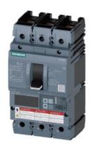
Circuit breaker 3VA6 UL frame 250 breaking capacity class C 100kA @ 480 V 3-pole, Line protection ETU860, LSIG, In=100A overload protection, 100% rated Ir=40A ...100A Short-circuit protection Isd=0.6..10x In, Ii=1.5..12x In N conductor protection optionally with external CT; up to 160% Ground-fault protection Ig=0.2... 1 x In, tg=0.05-0.8s nut keeper kit on both sides
