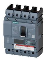
Circuit breaker 3VA6 UL frame 250 breaking capacity class C 100kA @ 480V 4-pole, Line protection ETU850, LSI, In=100A overload protection, 100% rated Ir=40A...100A Short-circuit protection Isd=0.6..10x In, Ii=1.5..12x In N conductor protection adjustable (OFF, up to 160%) without connection
