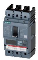
Circuit breaker 3VA6 UL frame 250 breaking capacity class C 100kA @ 480V 3-pole, Line protection ETU850, LSI, In=100A overload protection, 100% rated Ir=40A...100A Short-circuit protection Isd=0.6..10x In, Ii=1.5..12x In N conductor protection optionally with external CT, up to 160% without connection
