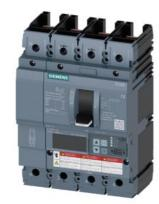
circuit breaker 3VA6 UL frame 250 breaking capacity class C 100kA @ 480V 4-pole, line protection ETU830, LIG, In=100A overload protection Ir=40A...100A short-circuit protection Ii=1.5...12 x In ground-fault protection Ig=0.2...1 x In, tg=0.05-0.8s without connection
