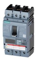
circuit breaker 3VA6 UL frame 250 breaking capacity class C 100kA @ 480 V 3-pole, line protection ETU830, LIG, ln=100A overload protection lr=40A ...100A short-circuit protection li=1.5...12 x ln ground-fault protection lg=0.2... 1 x ln, tg=0.05-0.8s cable connection on both sides
