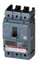
Circuit breaker 3VA6 UL frame 250 breaking capacity class C 100kA @ 480V 3-pole, Line protection ETU830, LIG, In=100A overload protection, 100% rated Ir=40A...100A Short-circuit protection Ii=1.5...12 x In Ground-fault protection Ig=0.2...1 x In, tg=0.05-0.8s without connection
