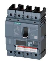
Circuit breaker 3VA6 UL frame 250 breaking capacity class C 100kA @ 480V 4pole, Line protection ETU556, LSI, In=100A overload protection, 100% rated Ir=40A...100A Short-circuit protection Isd=0.6..10x In, Ii=1.5..12x In N conductor protection adjustable (OFF, up to 160%) Ground-fault alarm message via EFB300 or COM without connection
