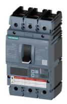
Circuit breaker 3VA6 UL frame 250 breaking capacity class C 100kA @ 480 V 3-pole, Line protection ETU556, LSI, In=100A overload protection, 100% rated Ir=40A ...100A Short-circuit protection Isd=0.6..10x In, Ii=1.5..12x In N conductor protection optionally with external CT; up to 160% Ground-fault alarm message via EFB300 or COM nut keeper kit on both sides
