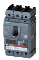
Circuit breaker 3VA6 UL frame 250 breaking capacity class C 100kA @ 480 V 3-pole, Line protection ETU560, LSIG, In=100A overload protection, 100% rated Ir=40A ...100A Short-circuit protection Isd=0.6..10x In, Ii=1.5..12x In N conductor protection optionally with external CT; up to 160% Ground-fault protection Ig=0.2... 1 x In, tg=0.05-0.8s nut keeper kit on both sides
