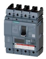
Circuit breaker 3VA6 UL frame 250 breaking capacity class C 100kA @ 480V 4-pole, Line protection ETU550, LSI, In=100A overload protection, 100% rated Ir=40A...100A Short-circuit protection Isd=0.6..10x In, Ii=1.5..12x In N conductor protection adjustable (OFF, up to 160%) without connection
