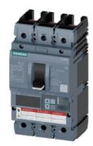
Circuit breaker 3VA6 UL frame 250 breaking capacity class C 100kA @ 480V 3-pole, Line protection ETU550, LSI, In=100A overload protection, 100% rated Ir=40A...100A Short-circuit protection Isd=0.6..10x In, Ii=1.5..12x In N conductor protection optionally with external CT, up to 160% without connection
