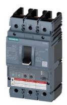
Circuit breaker 3VA6 UL frame 250 breaking capacity class C 100kA @ 480V 3-pole, Line protection ETU350, LSI, In=100A overload protection, 100% rated Ir=40A...100A Short-circuit protection Isd=1.5...10 x Ir, Ii=12 x In without connection
