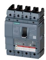
Circuit breaker 3VA6 UL frame 250 breaking capacity class C 100kA @ 480V 4pole, Line protection ETU320, LI, In=100A overload protection, 100% rated Ir=40A...100A Short-circuit protection Ii=1.5...12 x In N conductor protection adjustable (OFF, 50%, 100%) without connection
