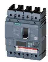
Circuit breaker 3VA6 UL frame 250 breaking capacity class H 65kA @ 480V 4pole, Line protection ETU856, LSI, In=100A overload protection, 100% rated Ir=40A...100A Short-circuit protection Isd=0.6..10x In, Ii=1.5..12x In N conductor protection adjustable (OFF, up to 160%) Ground-fault alarm message via EFB300 or COM without connection
