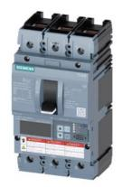
circuit breaker 3VA6 UL frame 250 breaking capacity class H 65kA @ 480 V 3-pole, line protection ETU856, LSI, In=100A overload protection Ir=40A ...100A short-circuit protection Isd=0.6..10x In, Ii=1.5..12x In N conductor protection opt. w. ext. CT; up to 160% ground-fault alarm message via EFB300 or COM cable connection on both sides
