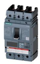
Circuit breaker 3VA6 UL frame 250 breaking capacity class H 65kA @ 480V 3pole, Line protection ETU856, LSI, In=100A overload protection, 100% rated Ir=40A...100A Short-circuit protection Isd=0.6..10x In, Ii=1.5..12x In N conductor protection optionally with external CT, up to 160% Ground-fault alarm message via EFB300 or COM without connection
