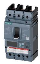
circuit breaker 3VA6 UL frame 250 breaking capacity class H 65kA @ 480V 3-pole, line protection ETU856, LSI, In=100A overload protection Ir=40A...100A shortcircuit protection Isd=0.6..10x In, Ii=1.5..12x In N conductor protection optionally with external current transformer, up to 160% ground-fault alarm message via EFB300 or COM without connection
