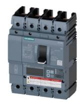
Circuit breaker 3VA6 UL frame 250 breaking capacity class H 65kA @ 480V 4-pole, Line protection ETU860, LSIG, In=100A overload protection, 100% rated Ir=40A...100A Short-circuit protection Isd=0.6..10x In, Ii=1.5..12x In N conductor protection adjustable (OFF, up to 160%) Ground-fault protection Ig=0.2...1 x In= tg=0.05-0.8s without connection
