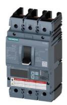
Circuit breaker 3VA6 UL frame 250 breaking capacity class H 65kA @ 480V 3-pole, Line protection ETU860, LSIG, In=100A overload protection, 100% rated Ir=40A...100A Short-circuit protection Isd=0.6..10x In, Ii=1.5..12x In N conductor protection optionally with external CT, up to 160% Ground-fault protection Ig=0.2...1 x In, tg=0.05-0.8s without connection
