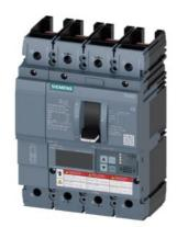
Circuit breaker 3VA6 UL frame 250 breaking capacity class H 65kA @ 480V 4-pole, Line protection ETU850, LSI, In=100A overload protection, 100% rated Ir=40A...100A Short-circuit protection Isd=0.6..10x In, Ii=1.5..12x In N conductor protection adjustable (OFF, up to 160%) without connection
