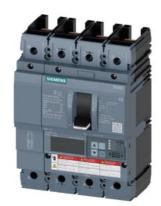
Circuit breaker 3VA6 UL frame 250 breaking capacity class H 65kA @ 480V 4-pole, Line protection ETU830, LIG, In=100A overload protection, 100% rated Ir=40A...100A Short-circuit protection Ii=1.5...12 x In Ground-fault protection Ig=0.2...1 x In, tg=0.05-0.8s without connection
