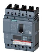
circuit breaker 3VA6 UL frame 250 breaking capacity class H 65kA @ 480V 4-pole, line protection ETU830, LIG, In=100A overload protection Ir=40A...100A short-circuit protection Ii=1.5...12 x In ground-fault protection Ig=0.2...1 x In, tg=0.05-0.8s without connection
