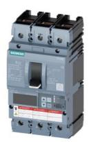
Circuit breaker 3VA6 UL frame 250 breaking capacity class H 65kA @ 480 V 3-pole, Line protection ETU830, LIG, In=100A overload protection, 100% rated Ir=40A ...100A Short-circuit protection li=1.5...12 x In Ground-fault protection lg=0.2... 1 x In, tg=0.05-0.8s cable connection on both sides
