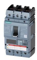
circuit breaker 3VA6 UL frame 250 breaking capacity class H 65kA @ 480 V 3-pole, line protection ETU830, LIG, In=100A overload protection Ir=40A ...100A short-circuit protection Ii=1.5...12 x In ground-fault protection Ig=0.2... 1 x In, tg=0.05-0.8s cable connection on both sides
