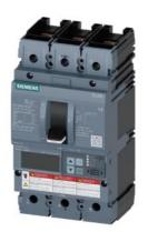
Circuit breaker 3VA6 UL frame 250 breaking capacity class H 65kA @ 480 V 3-pole, Line protection ETU830, LIG, In=100A overload protection, 100% rated Ir=40A ...100A Short-circuit protection li=1.5...12 x In Ground-fault protection lg=0.2... 1 x In, tg=0.05-0.8s nut keeper kit on both sides
