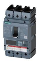
circuit breaker 3VA6 UL frame 250 breaking capacity class H 65kA @ 480 V 3-pole, line protection ETU830, LIG, ln=100A overload protection lr=40A ...100A short-circuit protection li=1.5...12 x In ground-fault protection lg=0.2... 1 x In, tg=0.05-0.8s nut keeper kit on both sides
