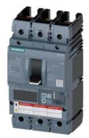
Circuit breaker 3VA6 UL frame 250 breaking capacity class H 65kA @ 480V 3-pole, Line protection ETU830, LIG, In=100A overload protection, 100% rated Ir=40A...100A Short-circuit protection Ii=1.5...12 x In Ground-fault protection Ig=0.2...1 x In, tg=0.05-0.8s without connection
