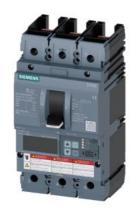
circuit breaker 3VA6 UL frame 250 breaking capacity class H 65kA @ 480V 3-pole, line protection ETU830, LIG, In=100A overload protection Ir=40A...100A short-circuit protection Ii=1.5...12 x In ground-fault protection Ig=0.2...1 x In, tg=0.05-0.8s without connection
