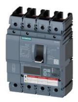
Circuit breaker 3VA6 UL frame 250 breaking capacity class H 65kA @ 480V 4-pole, Line protection ETU556, LSI, In=100A overload protection, 100% rated Ir=40A...100A Short-circuit protection Isd=0.6..10x In, Ii=1.5..12x In N conductor protection adjustable (OFF, up to 160%) Ground-fault alarm message via EFB300 or COM without connection
