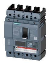
Circuit breaker 3VA6 UL frame 250 breaking capacity class H 65kA @ 480V 4-pole, Line protection ETU550, LSI, In=100A overload protection, 100% rated Ir=40A...100A Short-circuit protection Isd=0.6..10x In, Ii=1.5..12x In N conductor protection adjustable (OFF, up to 160%) without connection
