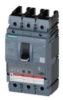
Circuit breaker 3VA6 UL frame 250 breaking capacity class H 65kA @ 480V 3-pole, Line protection ETU350, LSI, In=100A overload protection, 100% rated Ir=40A...100A Short-circuit protection Isd=1.5...10 x Ir, Ii=12 x In without connection
